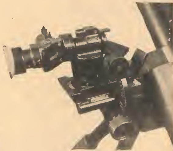
Figure 288. Panoramic sight for model 94 (1934) mortar has a 3\times magnification and a 13^\circ field of view. Micrometer drums enable readings to be made to the nearest mil.
