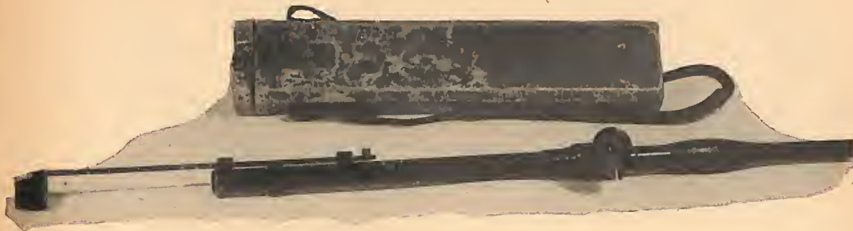
Figure 285. The hand held periscope, weighing 2.3 pounds, has a 5\times magnification and 10^\circ field of view.
