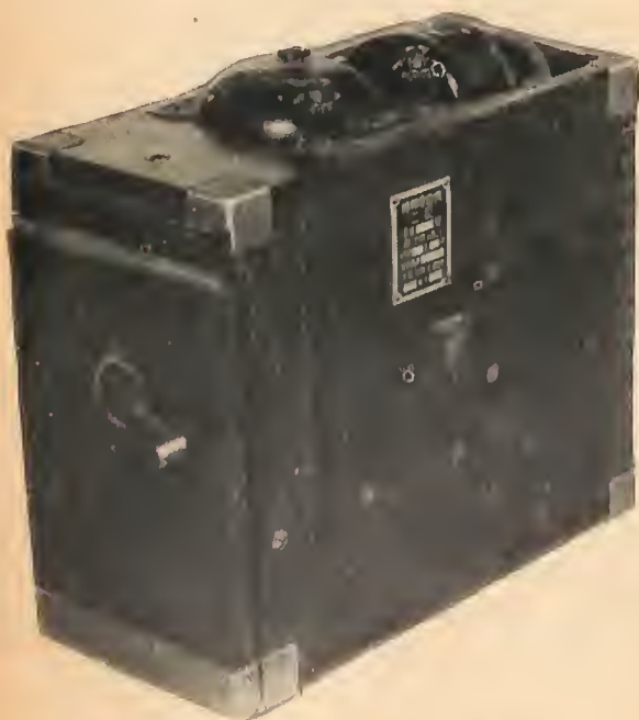
Figure 365. Model 2 trench telephone.
