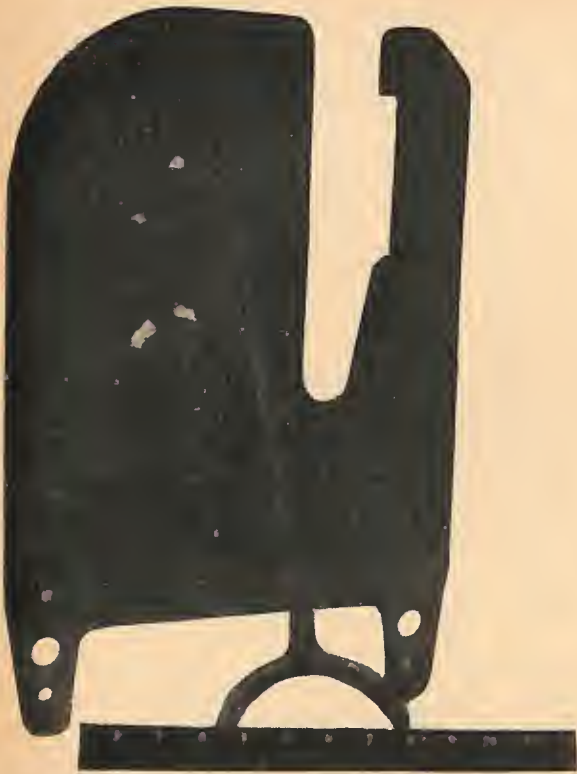
Figure 293. Rear of armor shield, size 14 in. x 20 in., showing penetration made with .30 cal. AP ammunition at 100 yards range and 30° angle of impact from normal.
