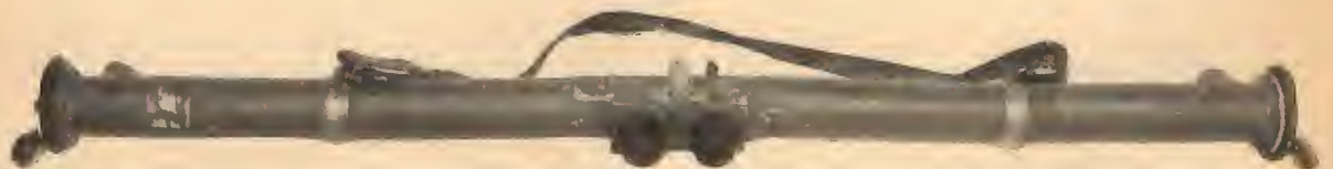
Figure 297. One meter base stereoscopic range finder. The reticle of this instrument is graduated from 250 to 6,000 (presumed to be meters). Markings indicate an 8\times magnification, a 4.5^\circ vertical and 5^\circ horizontal field of view.
