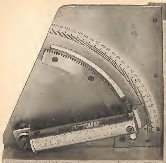
Figure 305. This gunner's quadrant is calibrated in units of 10 mils, extending from 0 to 1,410 mils (79°). A vernier scale enables adjustment to the nearest mil. It is considered possible that this quadrant has been designed primarily for use with the model 41 (1908) 75-mm infantry gun.
