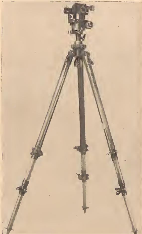
Figure 303. This aiming circle has a 4 \times magnification and a 10^\circ field of view. Similar to the American aiming circle, it is used by artillery units for measuring angles in azimuth and site, and for general topographical work.
