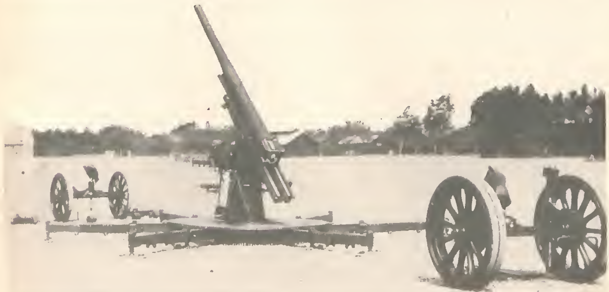
Figure 235. Model 14 (1925) 105-mm anti-aircraft gun showing detachable wheels used for transport of piece.
