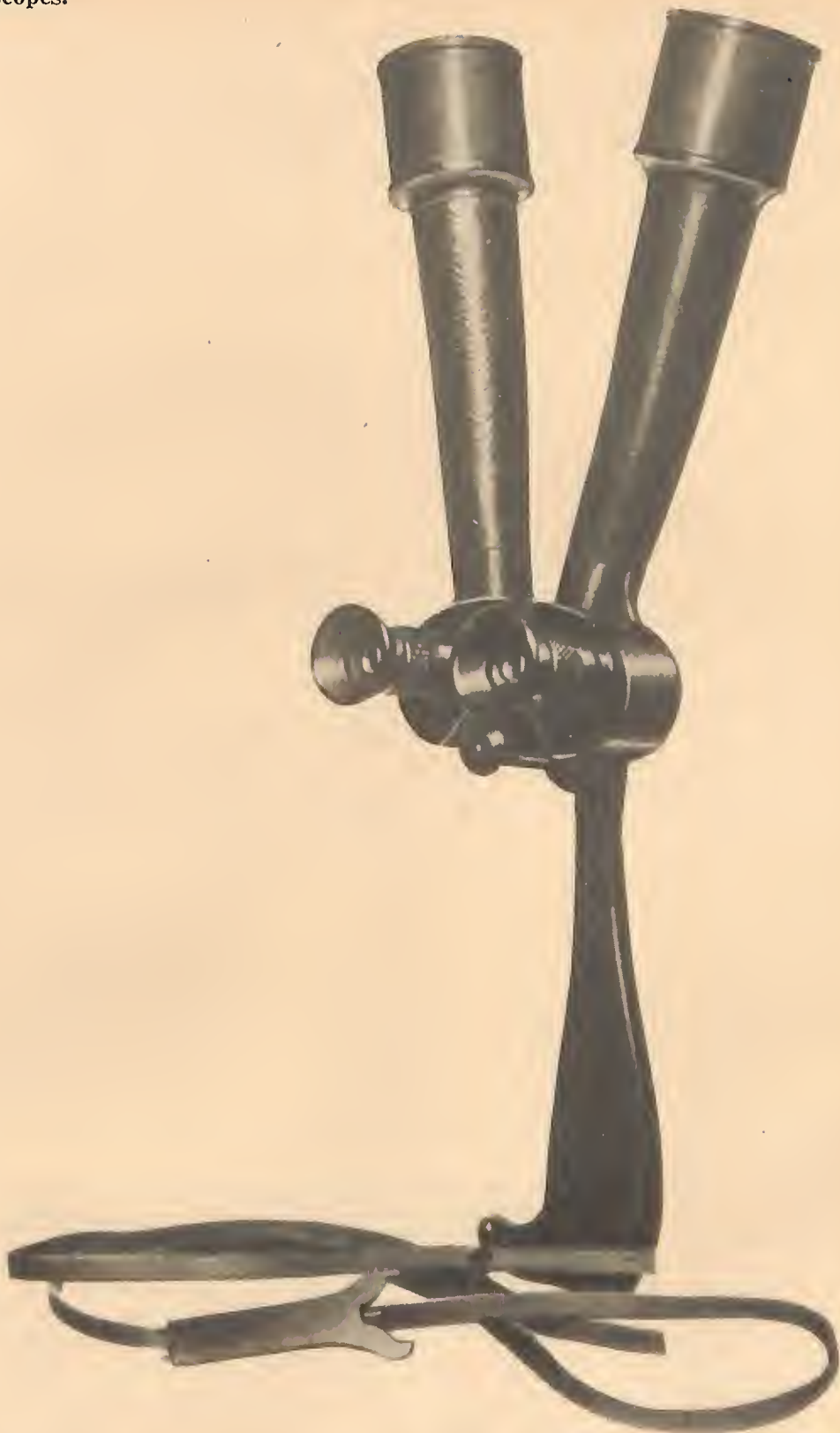
Figure 284. Periscope binocular, weighing 1.9 pounds, has a 10 × magnification and a 3° field of view.
