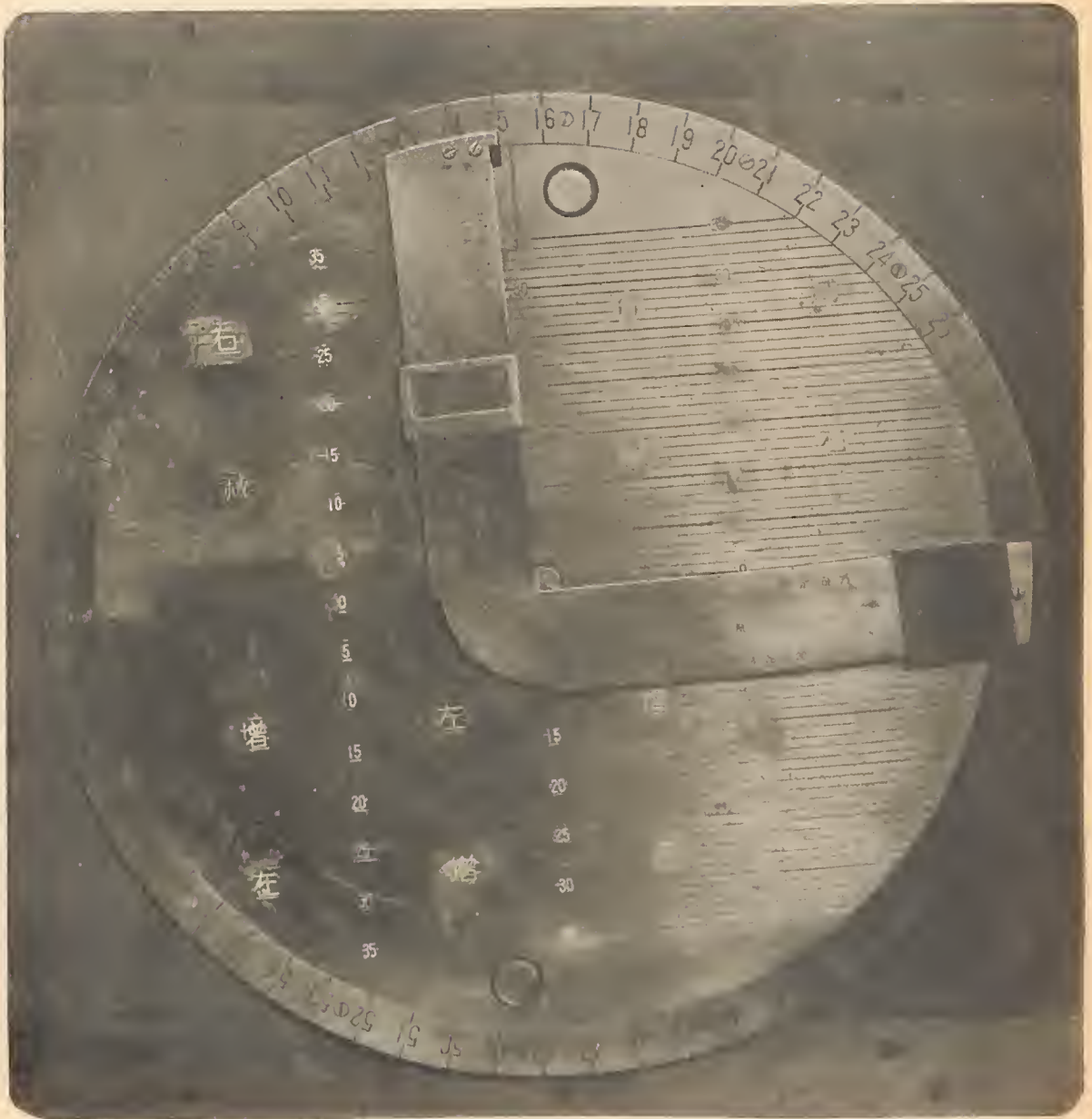
Figure 311. Powder-charge temperature and wind correction scale.
