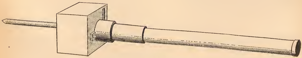
Figure 139. 70-mm barrage mortar showing spike and block used as base.
