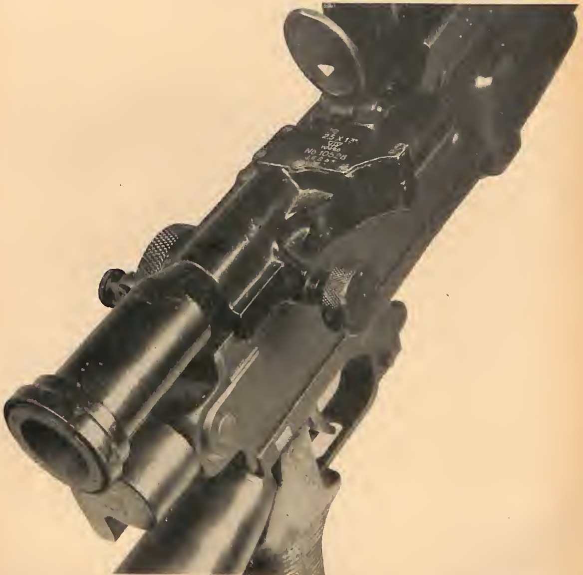
Figure 289. Telescopic sight for model 96 (1936) 6.5-mm light machine gun. The magnification is 2.5 X, the field of view is .13°, and the weight is 20 oz. The reticle (Graticule) pattern provides for drift and windage, and is calibrated for a maximum range of 1,500 meters (1,640 yards).
