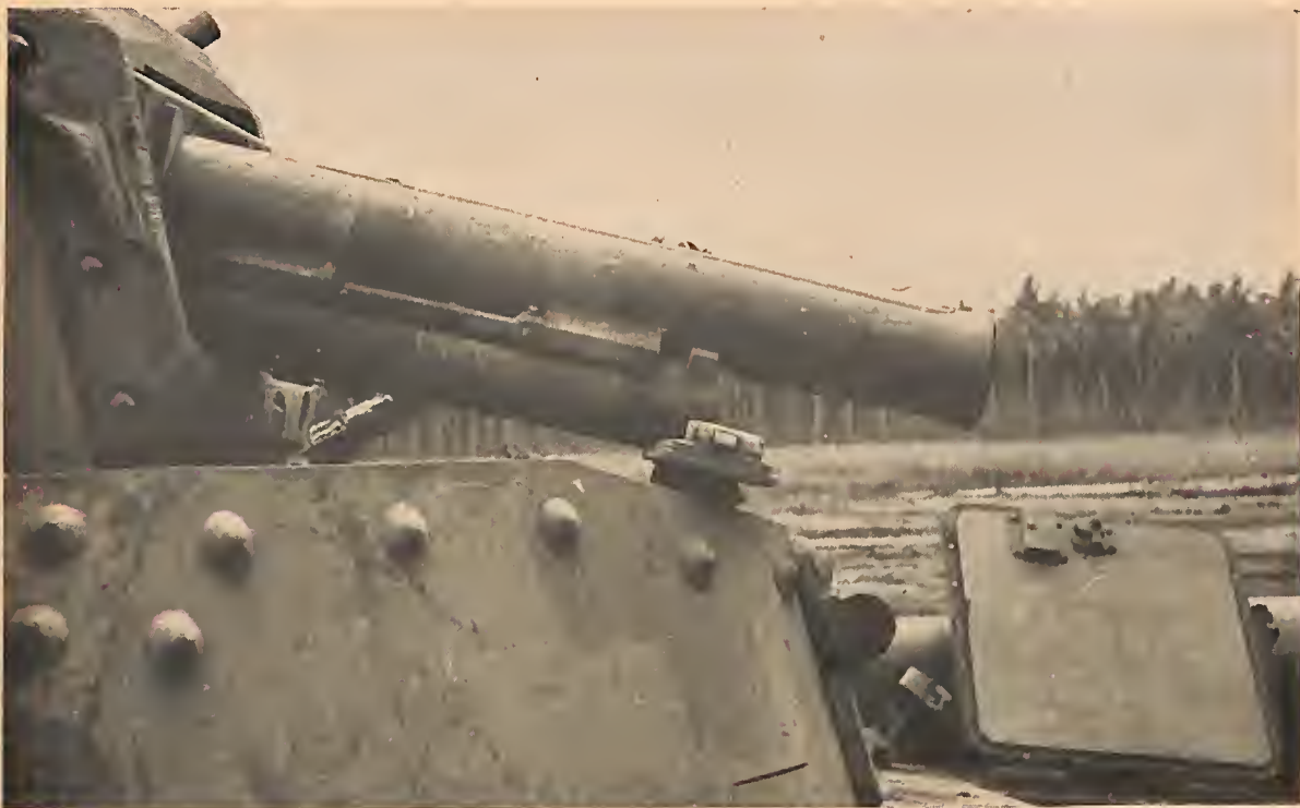
Figure 257. Model 97 (1937) 57-mm tank gun (showing its appearance from the outside of the turret).
