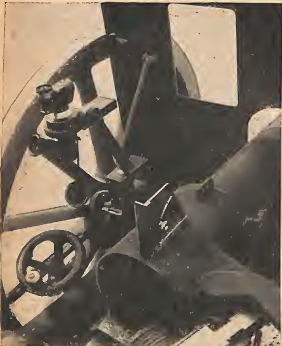
Figure 302. This panoramic sight appears to have been designed for use on more than one artillery piece. It is shown above mounted on the model 41 (1908) infantry gun. The sight has a 3 \times magnification and a 13^\circ field of view.
