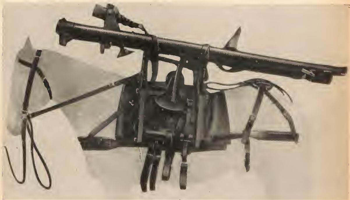
Figure 329. Trail of 75-mm infantry (mountain) gun disassembled and fastened to pack saddle.
