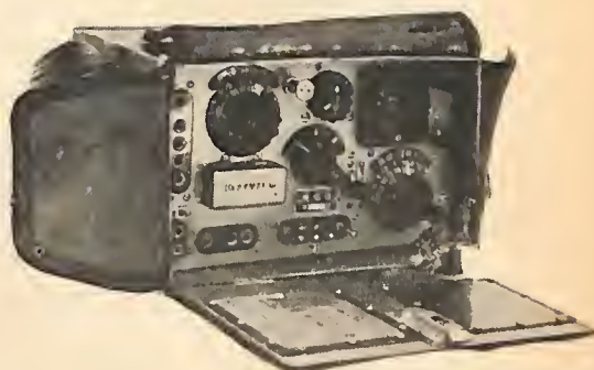
Figure 343. Model 94 Type 5. Transmitter-receiver Model 32. Transmitter. Operates CW or phone. Used with receiver shown below.
