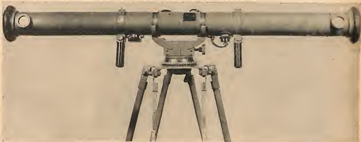
Figure 296. The 75-cm. base range finder is an inverted coincidence-type range finder with a 12\times magnification, a vertical field of view 2^\circ , and a 3^\circ horizontal field of view. It is calibrated to measure ranges up to 10,000 meters.
