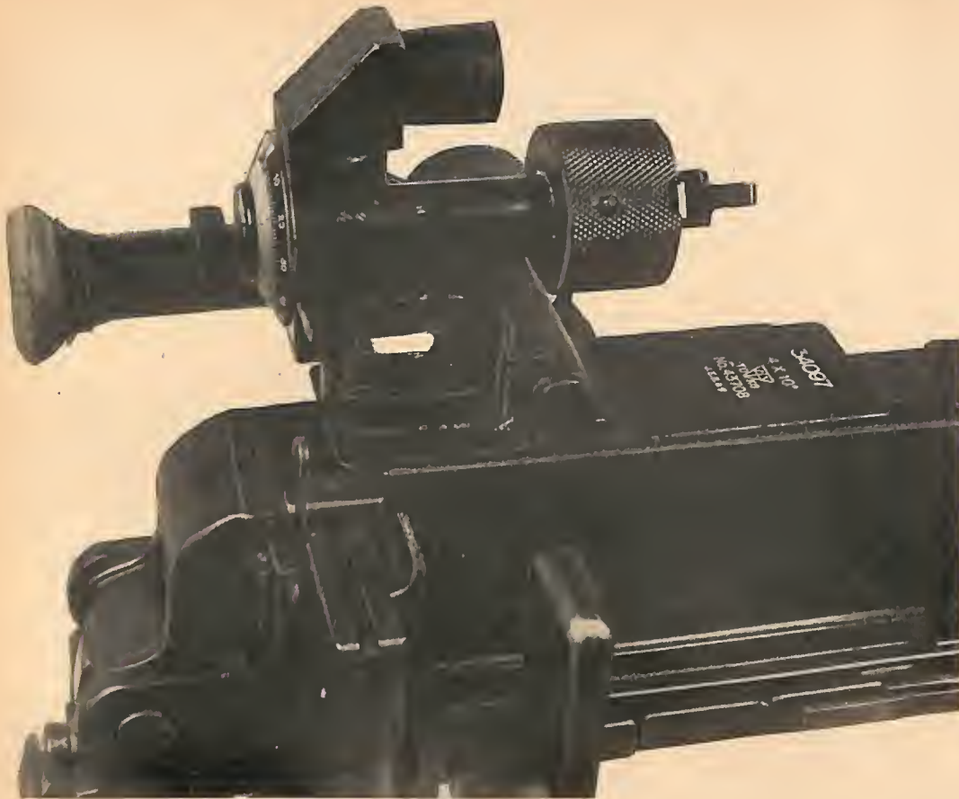
(Above) Figure 290. Telescopic sight for model 92 (1932) 7.7-mm machine gun has a 4\times magnification, a 10^\circ field of view, and a weight of 3 lbs., 6 ozs.
