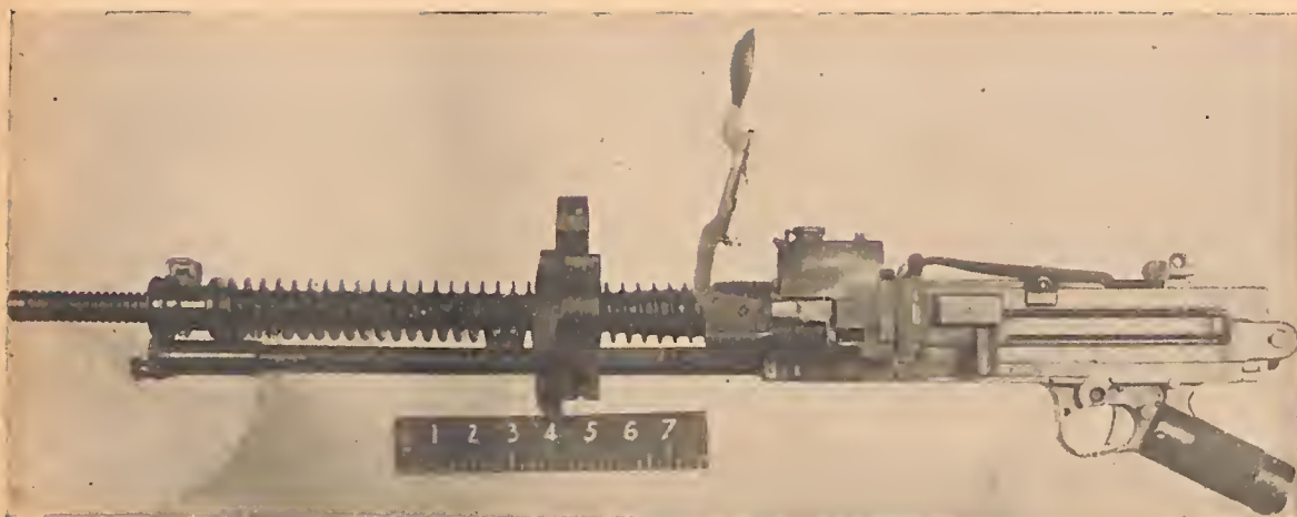
Figure 254. Model 91 (1931) 6.5-mm tank machine gun. Happer and butt are missing.
