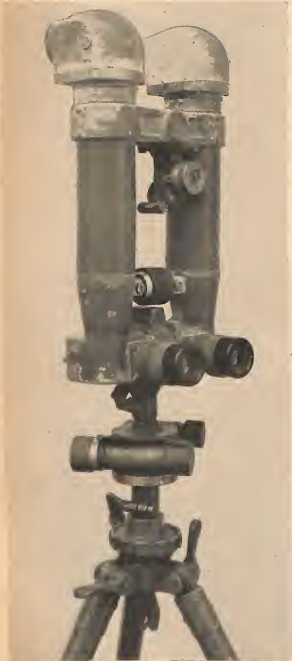
Figure 298. The model 93 battery commander's telescope permits measurement of angle of site from -300 to +300 mils, as well as measurement of azimuth. An unusual feature is that the telescopes cannot be placed in a horizontal plane for better stereoscopic vision. It has an 8\times magnification and a 6^\circ field of view.
