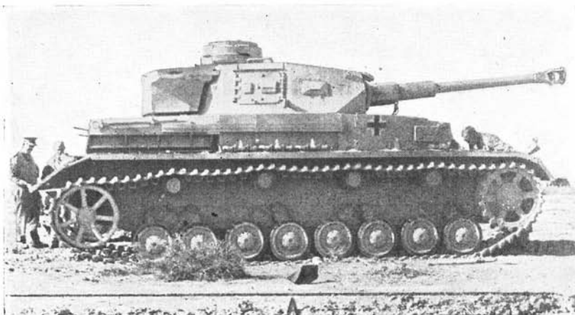
Figure 94.— Pz.Kw. IV (Sd.Kfz. 161) , medium tank, with long-barreled 75-mm high-velocity gun (equipped with double-baffle muzzle brake).
