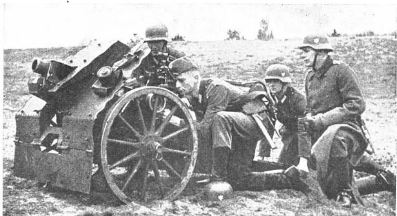
Figure 53.—75-mm infantry howitzer ( I.I.G. 18 ), horse-drawn. (This howitzer is also used by airborne units.)
