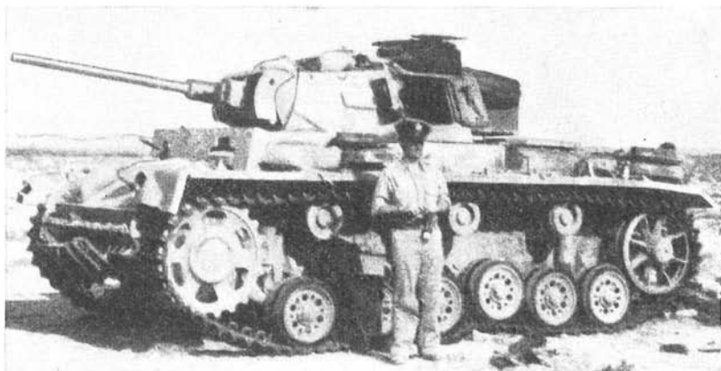
Figure 92.— Pz.Kw III (Sd.Kfz. 141) , medium tank, with long-barreled 50-mm gun.
