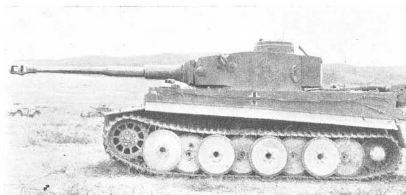
Figure 97.— Pz.Kw. VI , heavy tank, showing Christie-type bogie wheels.
