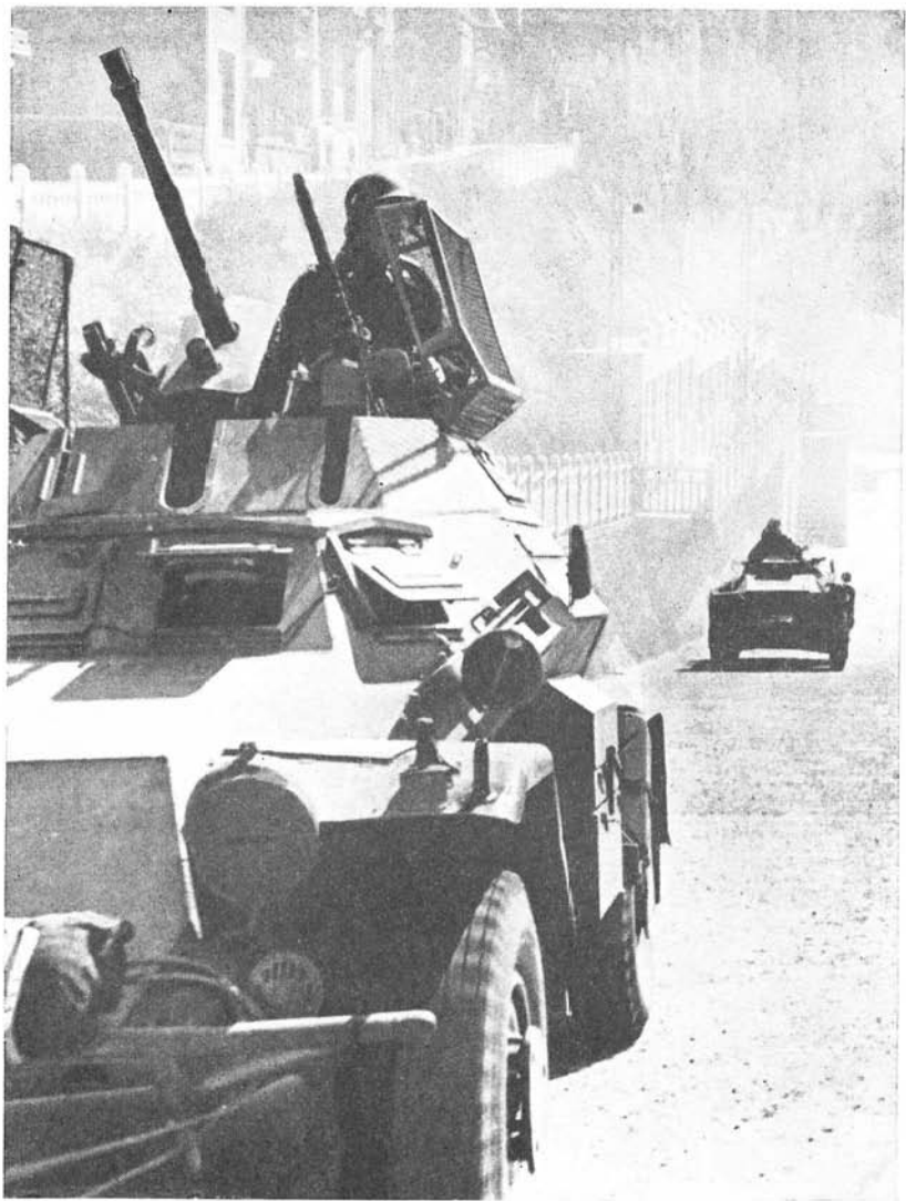
Figure 98.—Light armored car with 20-mm gun.
