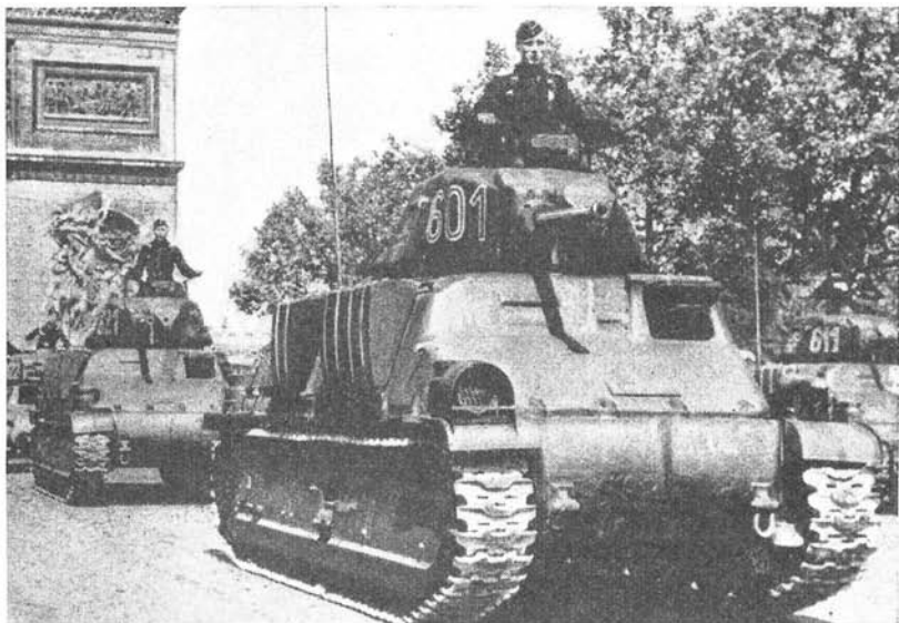
Figure 95.—18-ton Somua (captured French tank used by the Germans).
