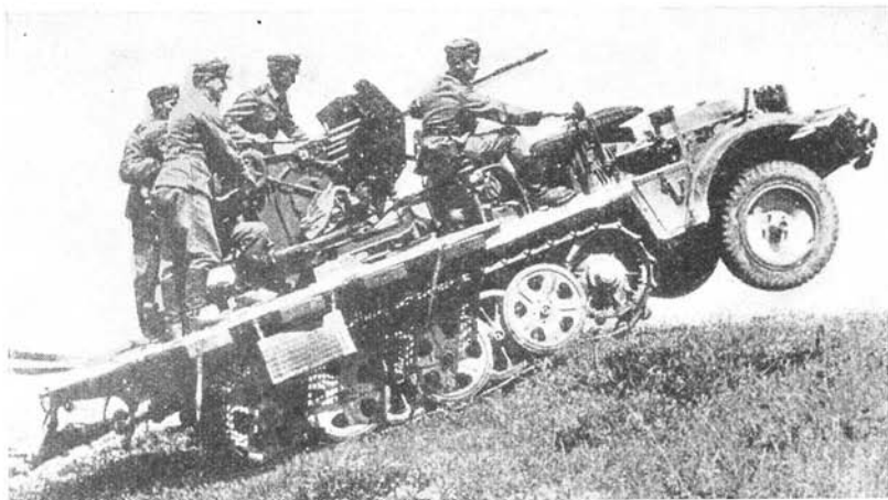
Figure 104.—20-mm dual-purpose gun.
