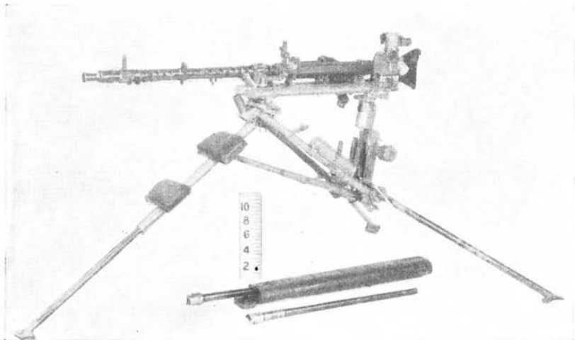
Figure 42.—7.92-mm heavy machine gun ( M.G. 34 ) on tripod mount.
