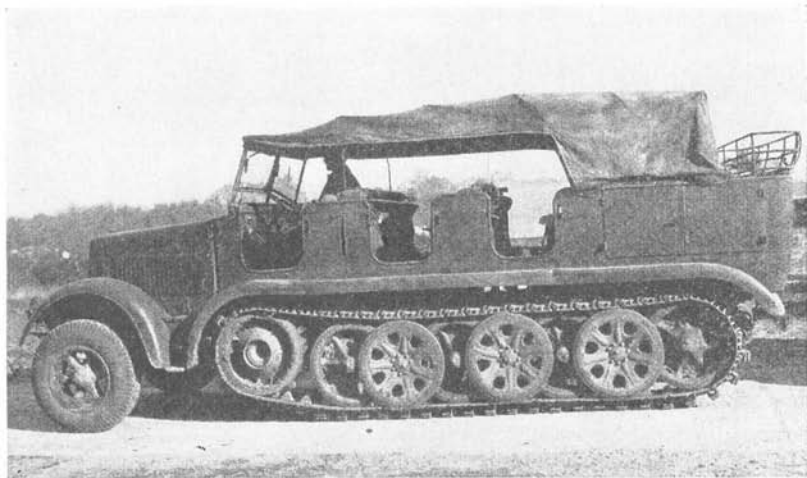
Figure 1.—Medium half-track tractor and prime mover, widely used to transport troops and tow weapons.
