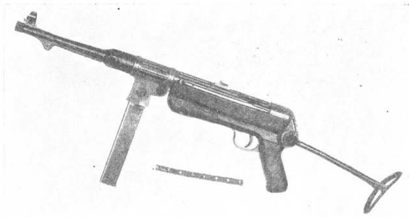
Figure 39.—9-mm submachine gun ( Schmeisser M.P. 38 ) with magazine attached and shoulder rest extended.
