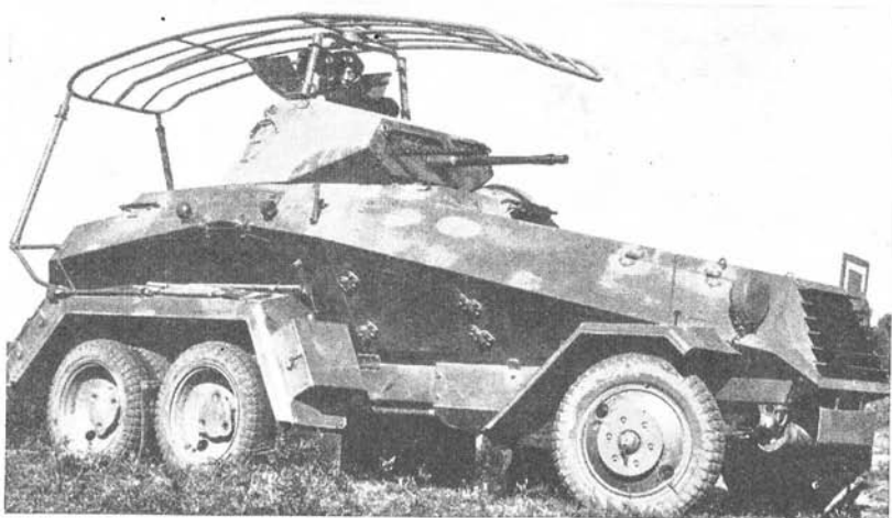
Figure 100.—Six-wheeled heavy armored car.
