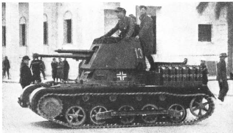
Figure 89.—Chassis of Pz.Kw. I used as mobile platform for Czech 47-mm antitank gun.
