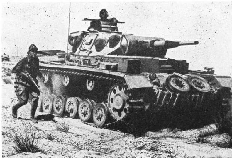
Figure 91.— Pz.Kw. III (Sd.Kfz. 141) , medium tank, with short-barreled 50-mm gun.
