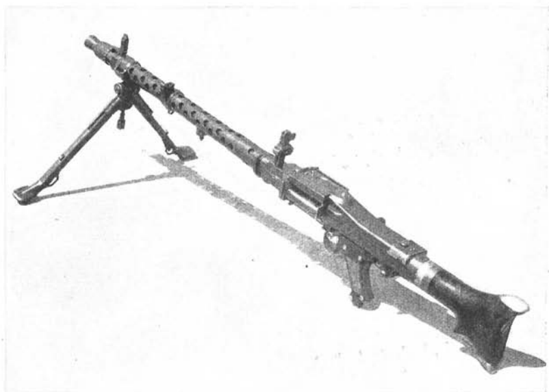
Figure 41.—7.92-mm light machine gun ( M.G. 34 ) on bipod mount.
