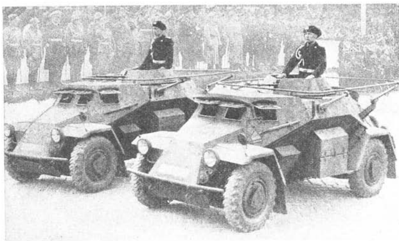
Figure 99.—Light armored car, showing machine-gun armament.
