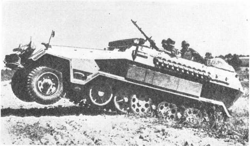
Figure 17.—Medium armored personnel carrier ( Sd.Kfz. 251 ).
