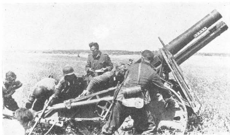
Figure 55.—150-mm infantry howitzer (s.I.G. 33) in firing position.
