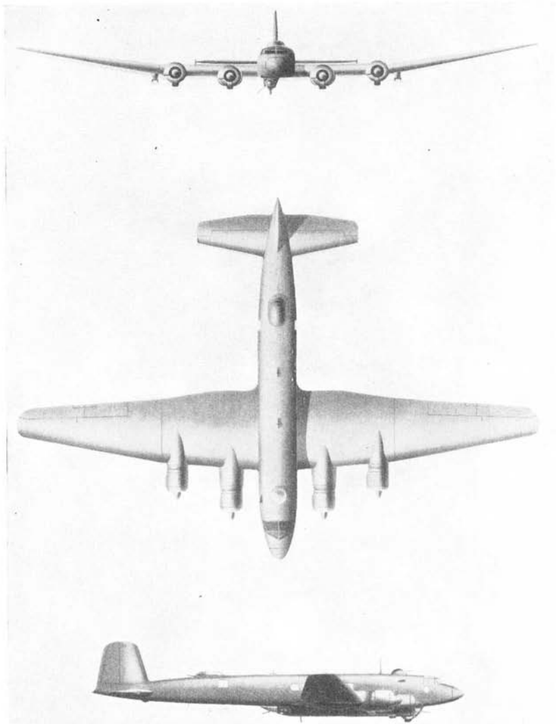
Figure 172.— Focke-Wulf 200 Kurier (four-engine heavy bomber, used for long-range bombing and attacks on Allied convoys).
