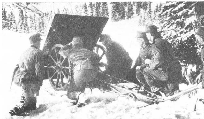
Figure 72.—75-mm mountain howitzer with shield.
