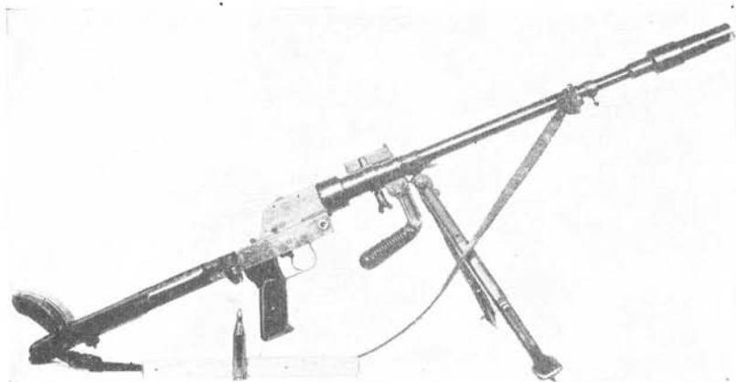
Figure 46.—7.92-mm antitank rifle ( Pz.B. 38 ) with grenade discharger.
