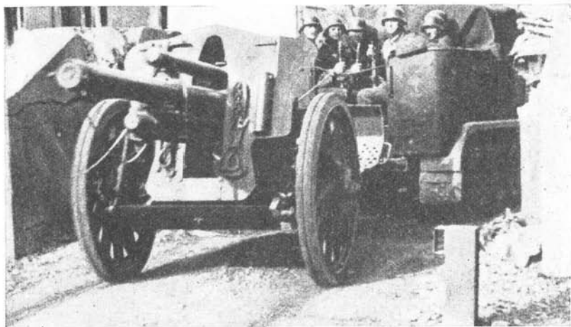
Figure 60.—105-mm gun-howitzer with half-track prime mover.
