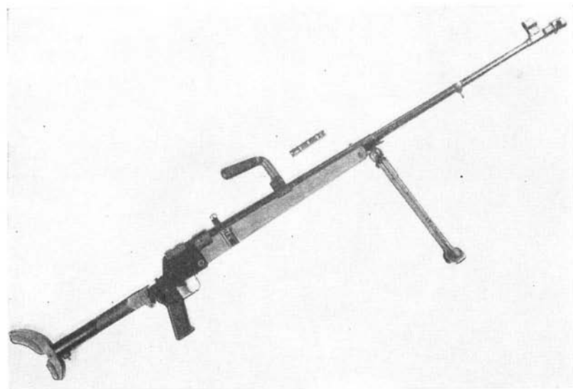
Figure 47.—7.92-mm antitank rifle ( Pz.B. 39 ) with stock and bipod extended.
