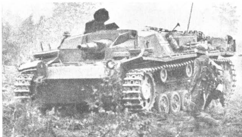
Figure 79.— Pz.Kw. III chassis mounted with 75-mm short-barreled assault gun.
