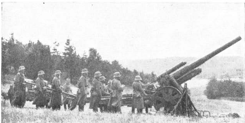
Figure 61.—150-mm gun-howitzer ( s.F.H. 18 ), horse-drawn, with crew, in firing position.
